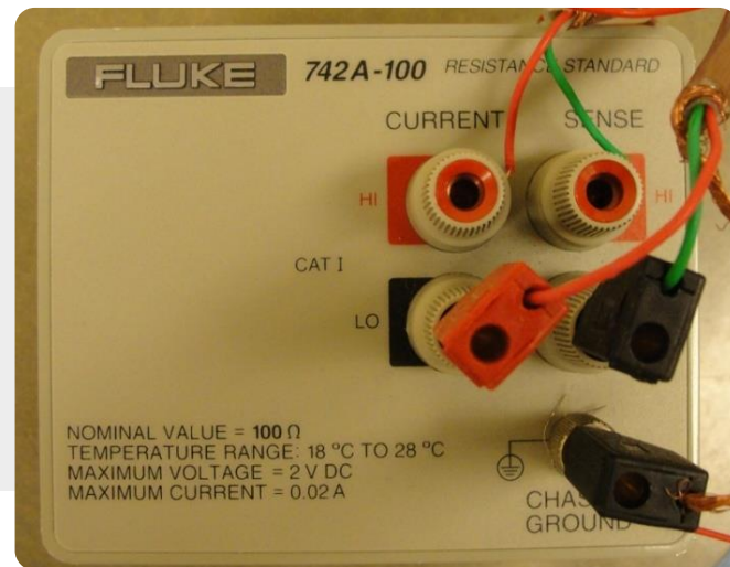
Fluke 742A-100 resistor (100 \Omega ) \alpha(23\text{ }^\circ\text{C}) \approx 4,00 \cdot 10^{-8} \text{ 1/K} \beta(23\text{ }^\circ\text{C}) \approx -2,60 \cdot 10^{-8} \text{ 1/K}^2
