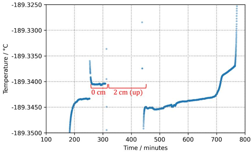
Figure 4 Plateau obtained in 250 to 270 minutes. Attempting to calibrate at immersion depths destabilized the system.
