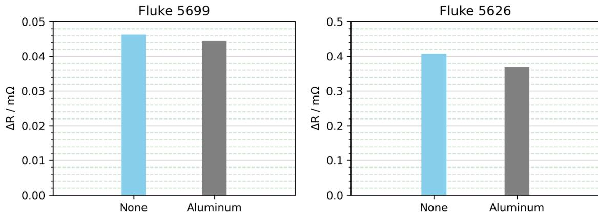
Figure 7 Self-heating in mΩ for SPRT Fluke 5699 and 5626 with aluminum bushing and without bushing.
