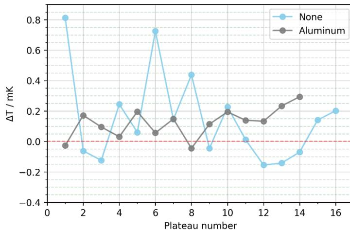
Figure 8 Temperature difference (ΔT) of freezing-melting argon plateau with aluminum bushing and without bushing.
