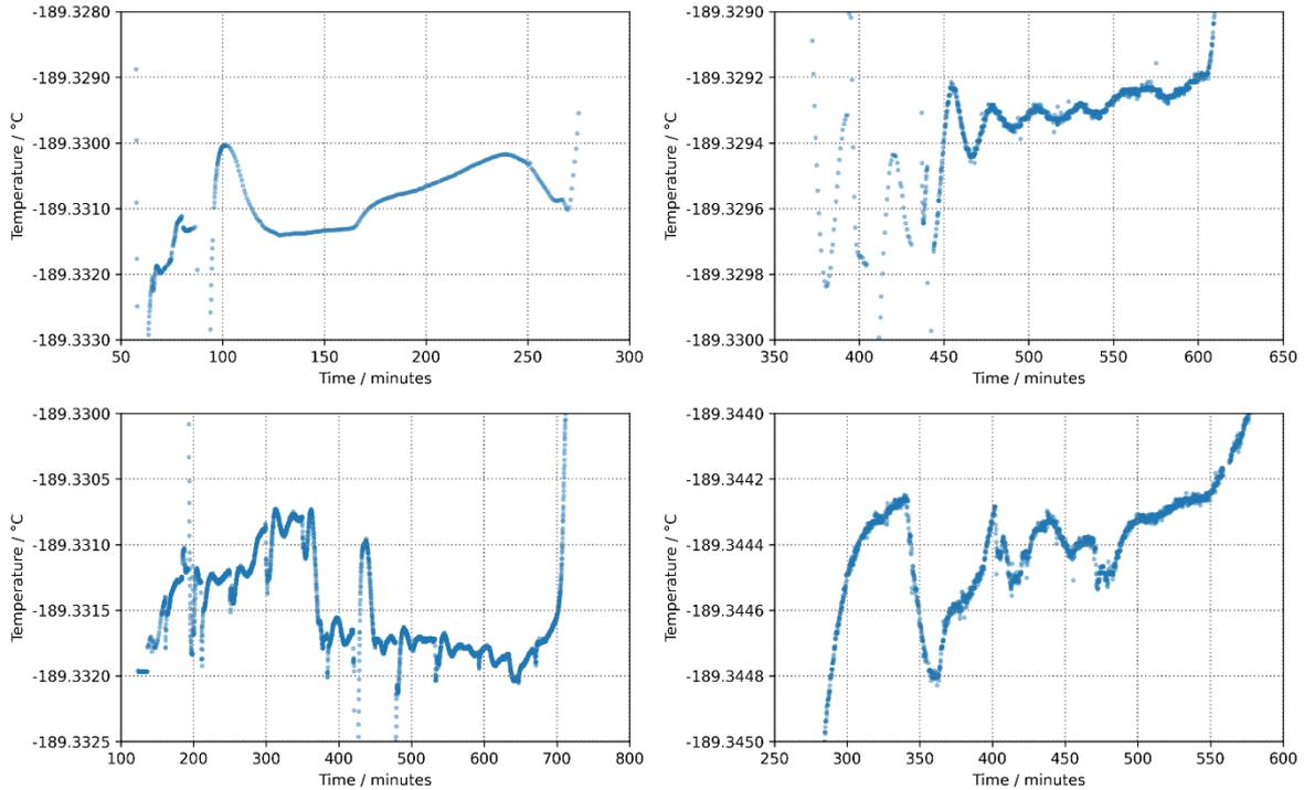
Figure 3 Failed plateaus of the performance of TP-Ar in its beginnings.
