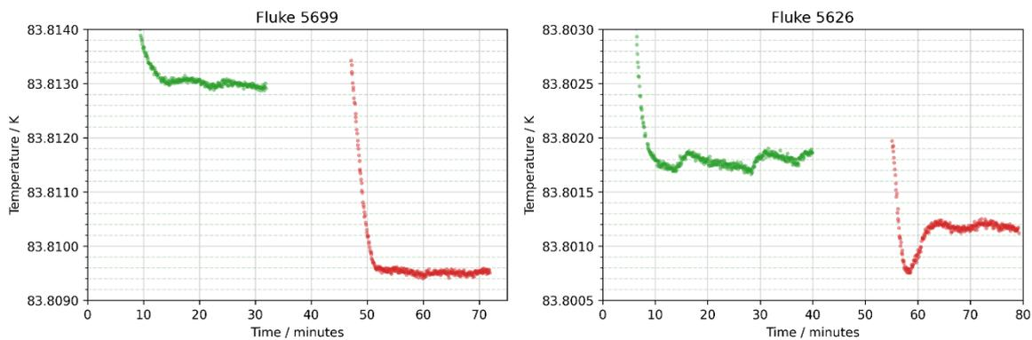
Figure 6 Immersion depth profiles of Fluke 5699 and Fluke 5626.
