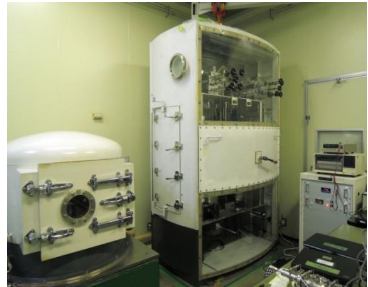
The balances of the static gravimetric system of NMIJ/AIST.
