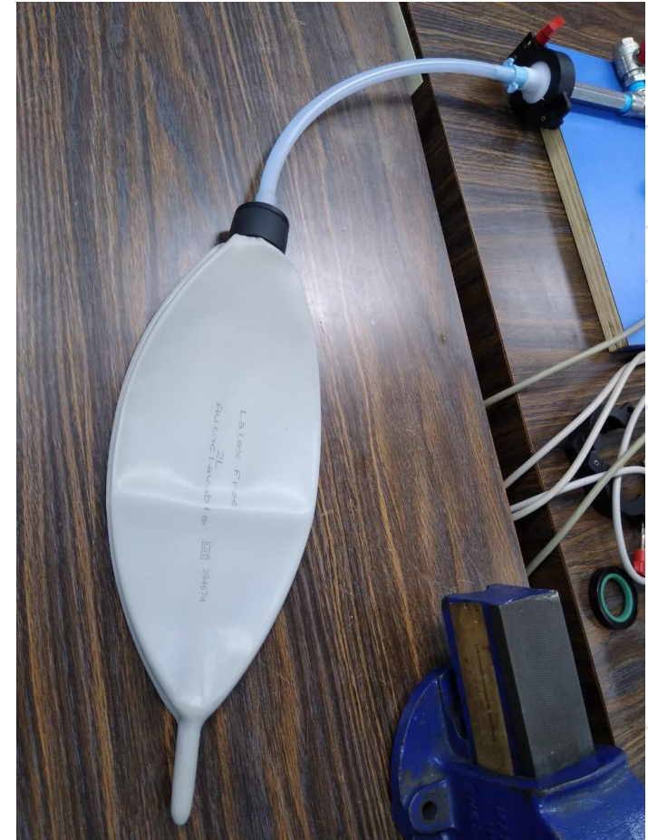
Test lung at LCM; compliance 18 mL/hPa
