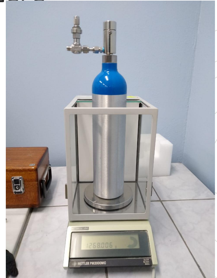
Weighting the gas cylinder
