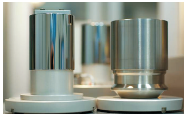
Fig 1. Piston (left) and cylinder (right) of a pressure standard piston-cylinder assembly. This model was custom-made for the Boltzmann constant project. The artefacts are mounted on clamping disks.
