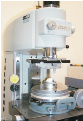
Fig. 2 Reference roundness measuring instrument Talyrond 73. The image shows the set-up for running the multi-step error separation procedure.
