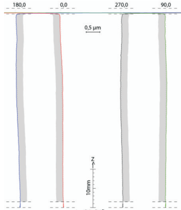
Fig. 13 Reference straightness profiles of the four generatrices 0^\circ , 90^\circ , 180^\circ and 270^\circ of the piston of assembly PCU 6222. The measurement was performed with the MFU8PTB in reversal mode.
