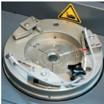
Fig. 10 MFU110WP rotary table with double pairs as kinematic bearing counterpart and quick-clamping mechanism for the clamping disks. The cables are connected to Pt100 resistance thermometers.
