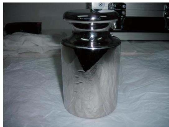
**Figure 1.** Damage sustained by a 2 kg mass piece shipped outside the region.
